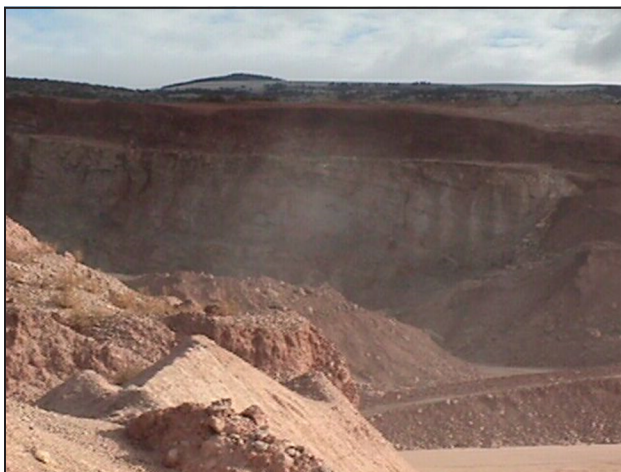
FIGURE 2.9 Failure to cleanly strip the overlying red Amsden Formation from underlying Madison Limestone results in Amsden material contaminating the Madison Limestone product
